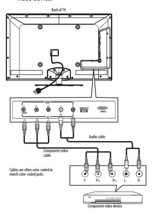
3 Connect an audio cable (not provided) to the AV/COMP L/R audio jacks on the back of your TV and to the L/R AUDIO OUT jacks on the component video device.
